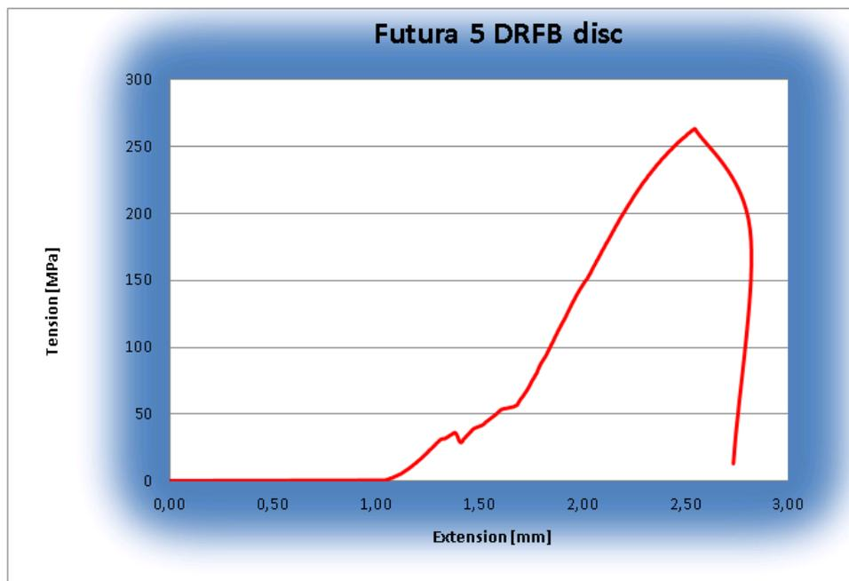
Figure 73: Graphic progress of 5<sup>th</sup> prototype DRFB disc crown tensile test
