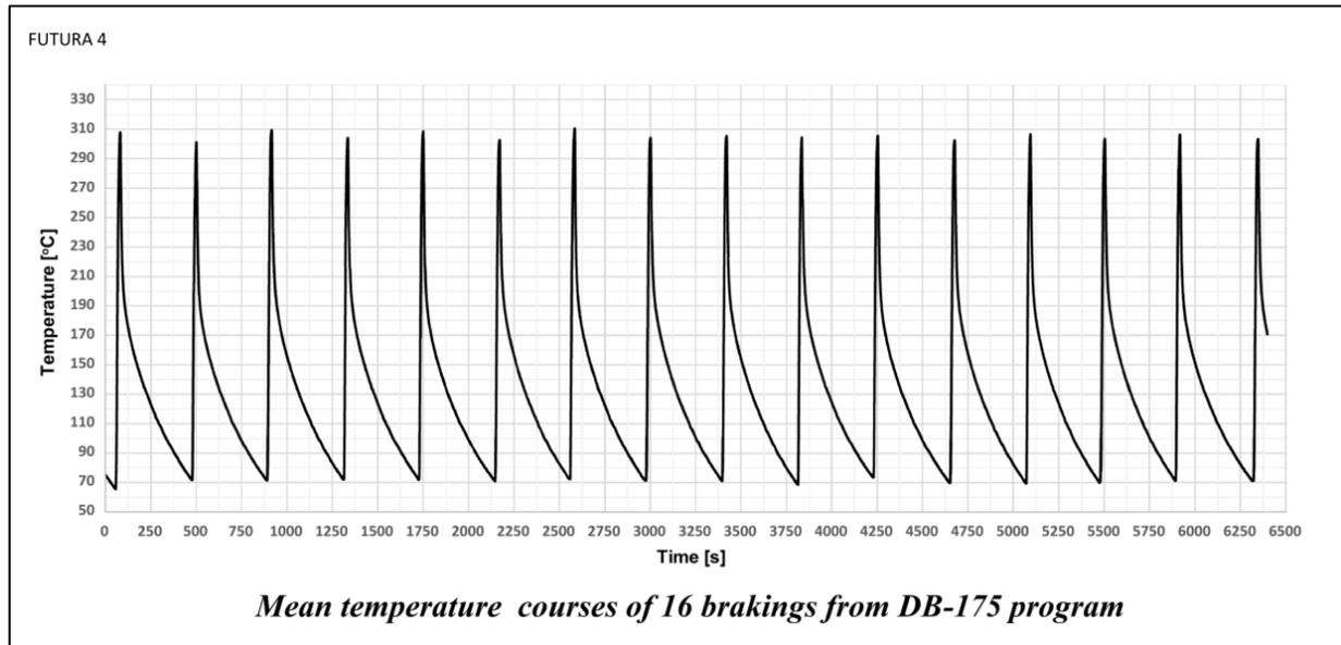
Figure 68: Temperatures of DRFB disc during DB-175 test
