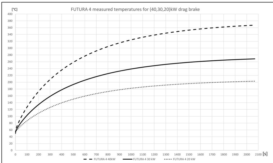
Figure 67: Temperatures of disc during heat dissipation test
