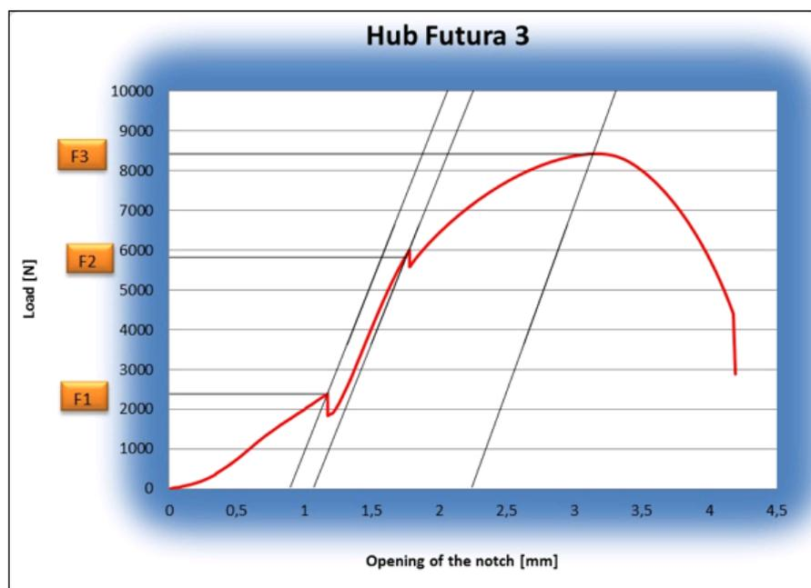
Figure 51: DRFB disc hub graphic fracture toughness test progress
