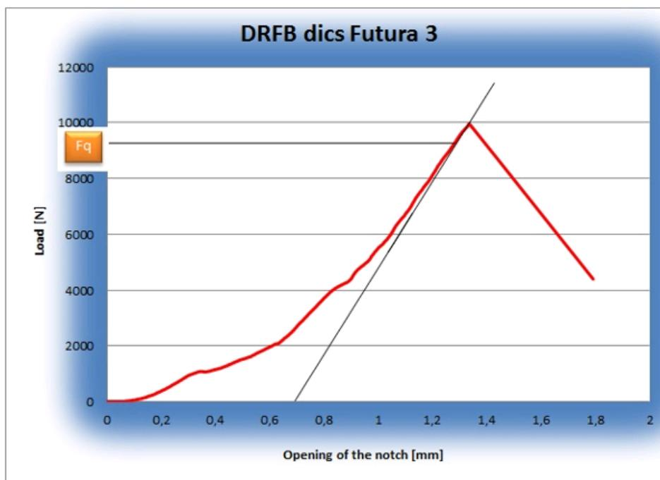
Figure 52: DRFB disc crown graphic fracture toughness progress
