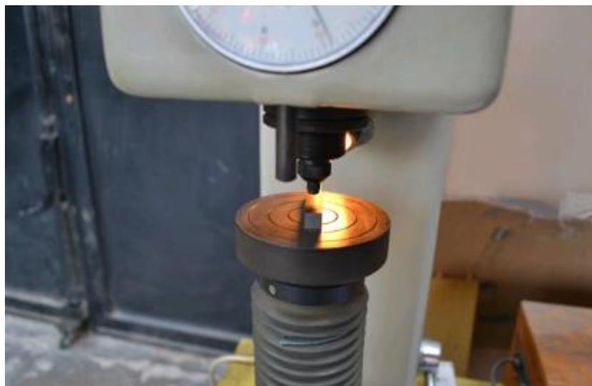
Figure 11: Hardness test process
