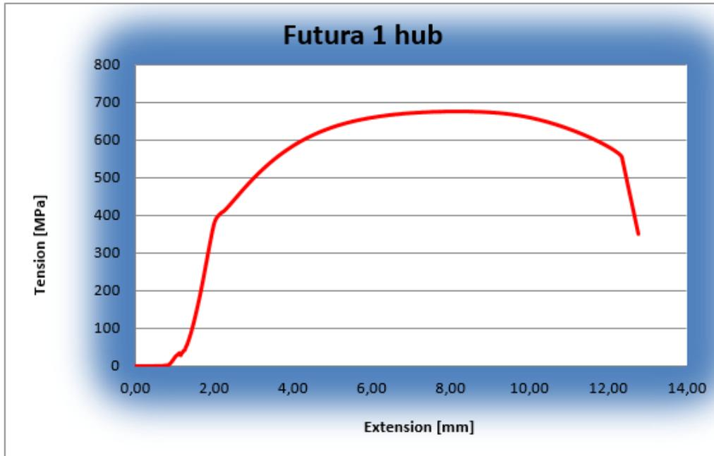
Figure 10: Graphic progress of 1<sup>st</sup> prototype DRFB disc hub tensile test
