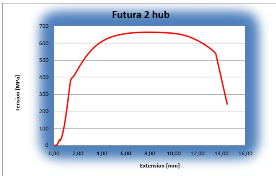
Figure 35: Graphic progress of 2<sup>nd</sup> prototype DRFB disc hub tensile test
