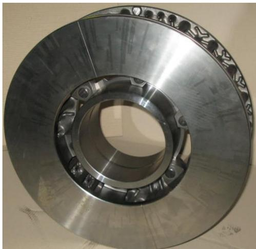
Figure 53: 3<sup>rd</sup> prototype DRFB disc
