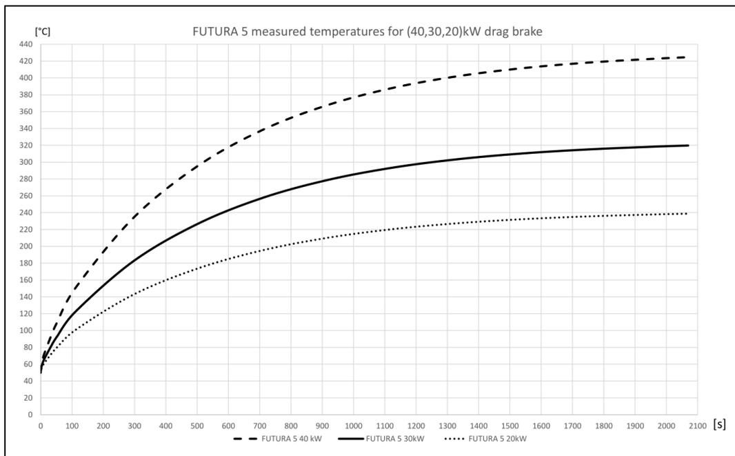
Figure 77: Temperatures of disc during heat dissipation test
