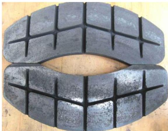
Figure 33: Brake pads after 2A2 test
