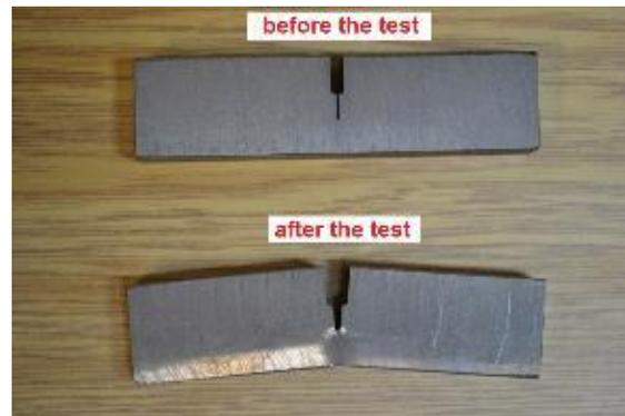
Figure 17: Fracture toughness test samples
