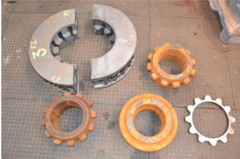
Figure 1: Samples of DRFB disc and hub
