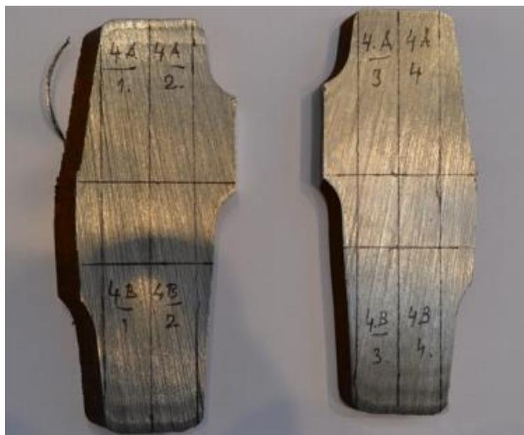
Figure 2: Cut samples of DRFB disc hub
