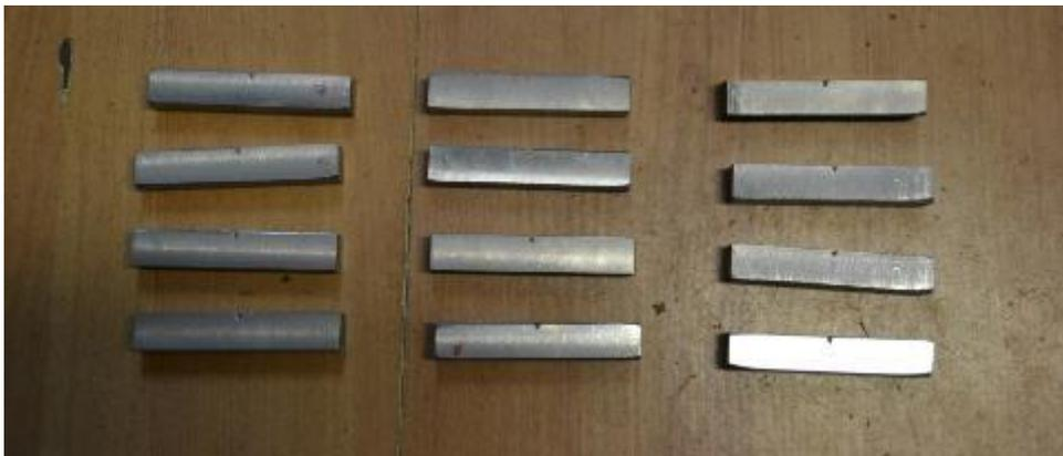
Figure 15: Charpy test samples
