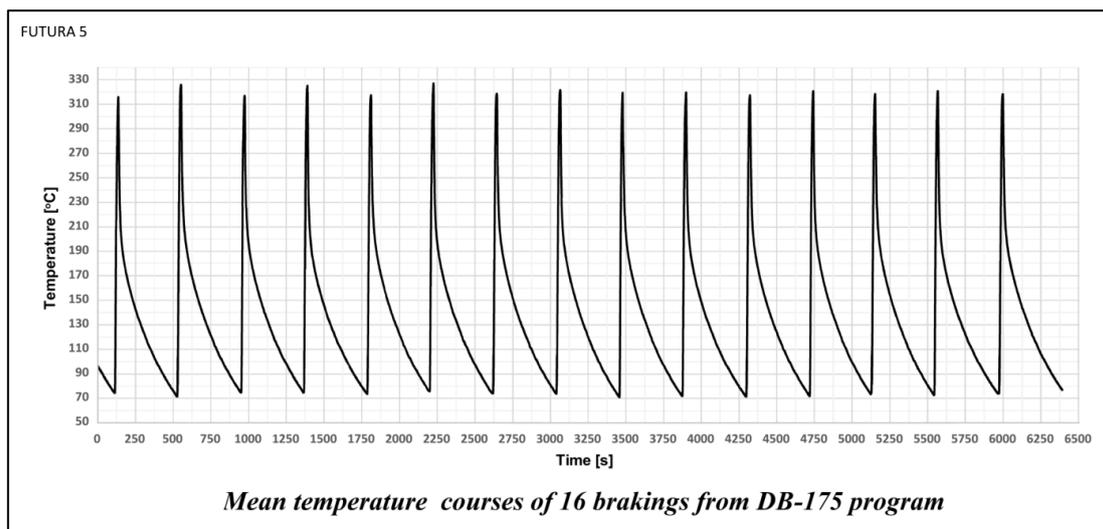
Figure 78: Temperatures of DRFB disc during DB-175 test
