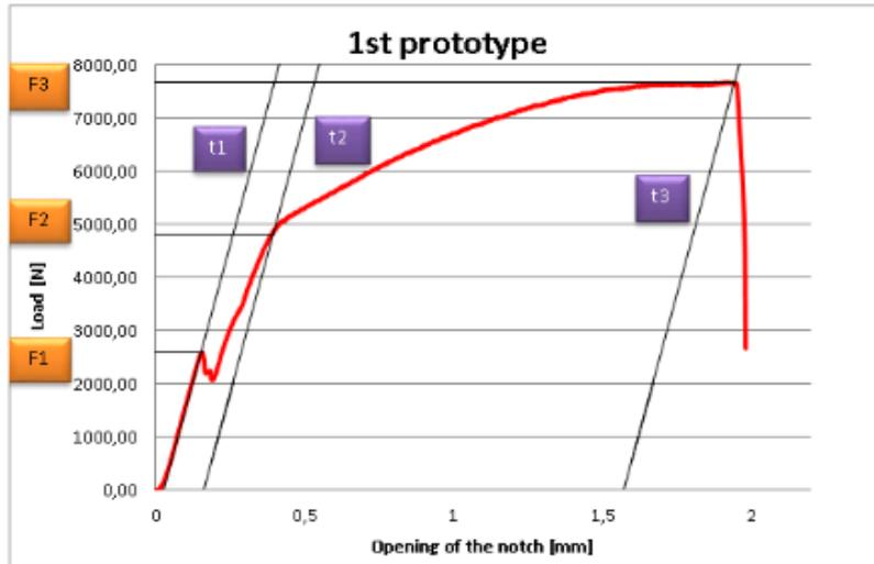
Figure 19: DRFB disc hub graphic fracture toughness progress
