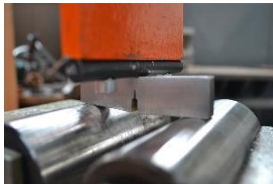
Figure 18: Fracture toughness test process
