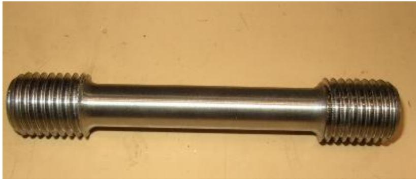
Figure 12: Fatigue material test sample
