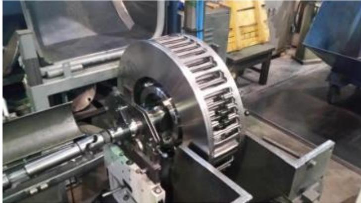
Figure 46: 2<sup>nd</sup> prototype vibration measurement
