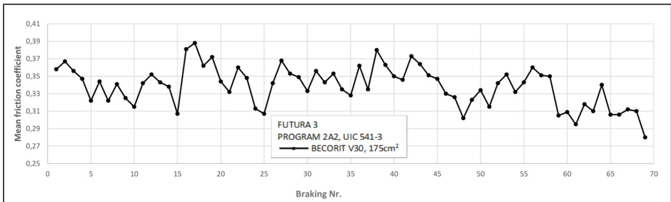
Figure 59: 3<sup>rd</sup> prototype friction coefficient (Program 2A2)
