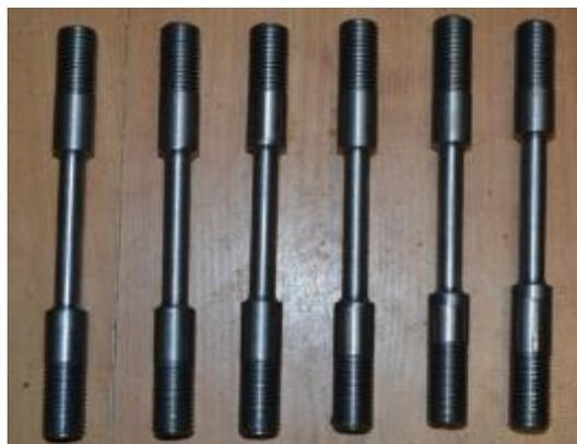
Figure 7: Tensile test machined samples
