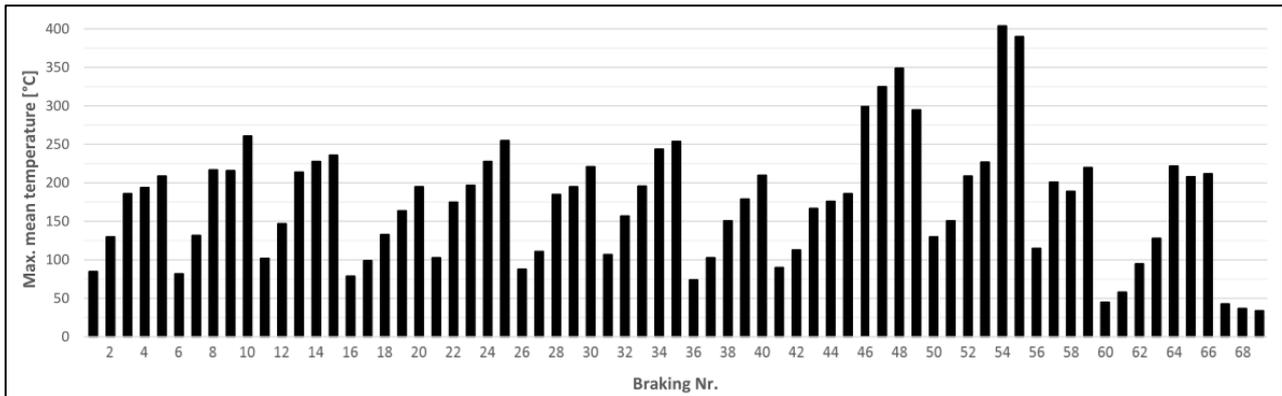
Figure 42: Temperatures of DRFB disc during 2A2 test program
