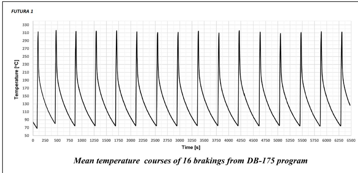
Figure 27: Temperatures of disc during DB-175 test
