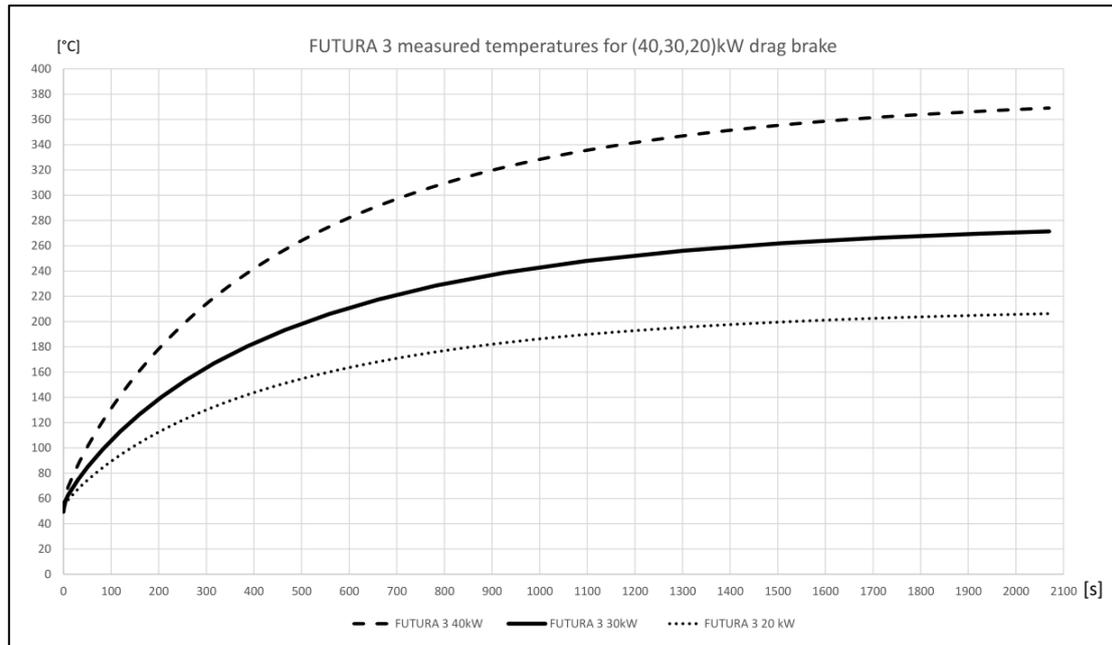
Figure 55: Temperatures of disc during heat dissipation test
