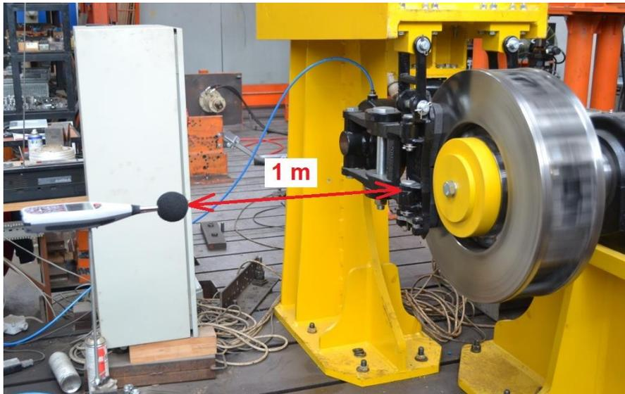
Figure 22: Position of microphone on test bench
