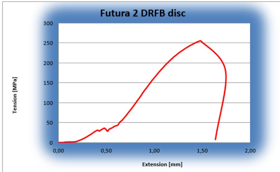
Figure 34: Graphic progress of 2<sup>nd</sup> prototype DRFB disc crown tensile test
