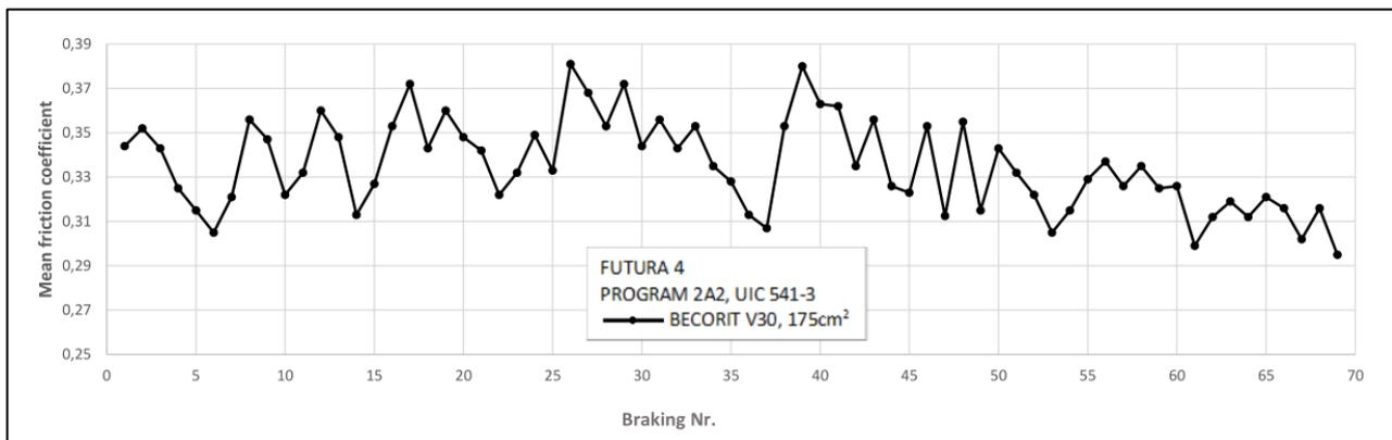
Figure 71: 4<sup>th</sup> prototype friction coefficient (Program 2A2)
