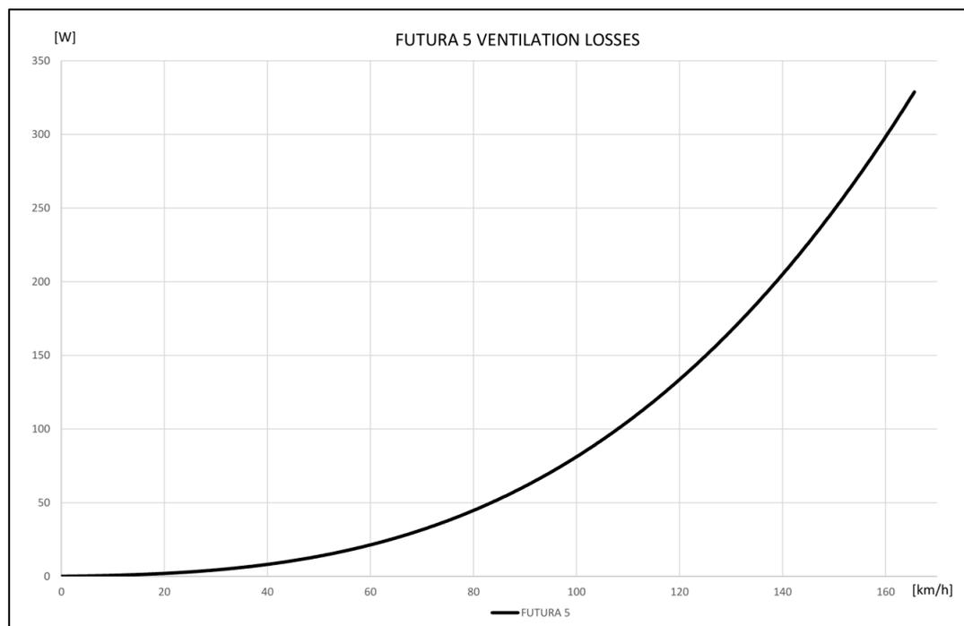
Figure 82: 5<sup>th</sup> prototype ventilation losses
