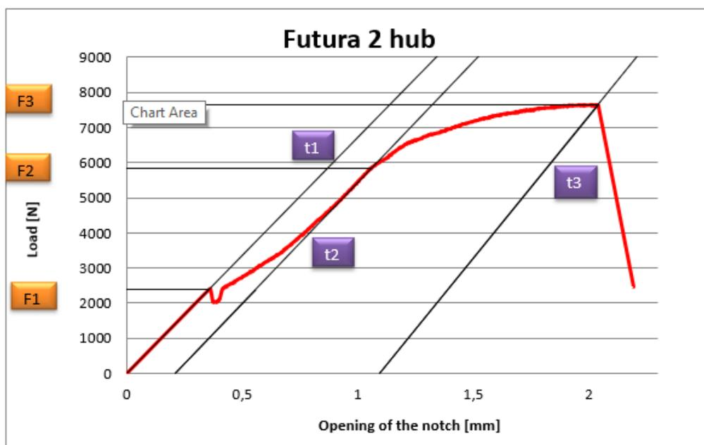
Figure 38: DRFB disc hub graphic fracture toughness test progress
