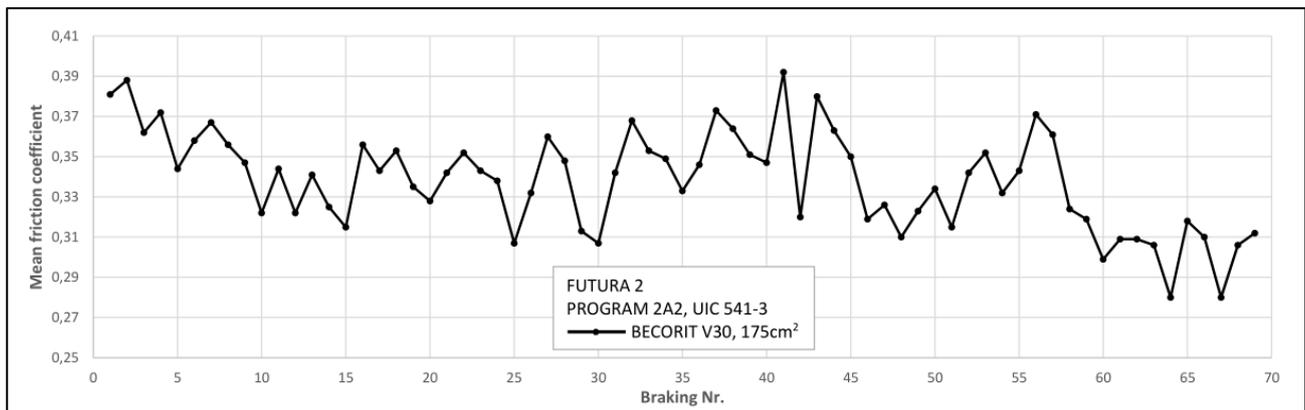
Figure 47: 2<sup>nd</sup> prototype friction coefficient (Program 2A2)
