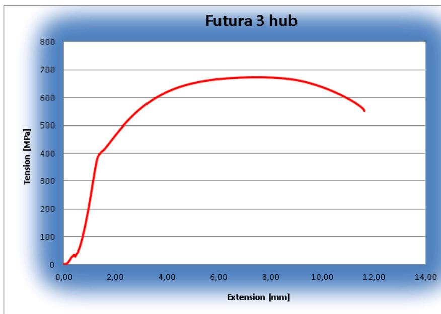
Figure 50: Graphic progress of 3<sup>rd</sup> prototype DRFB disc hub tensile test
