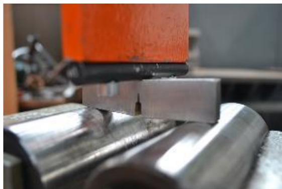
Figure 37: Fracture toughness test samples
