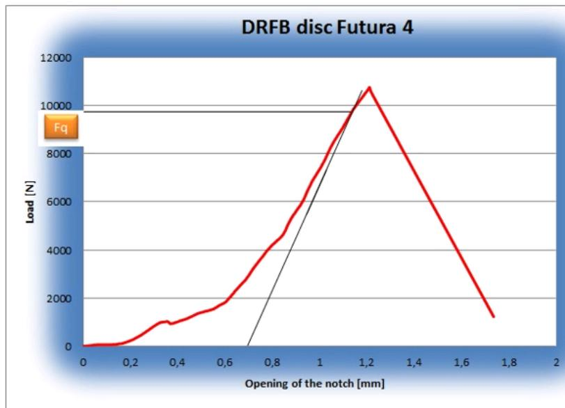
Figure 64: DRFB disc crown graphic fracture toughness progress
