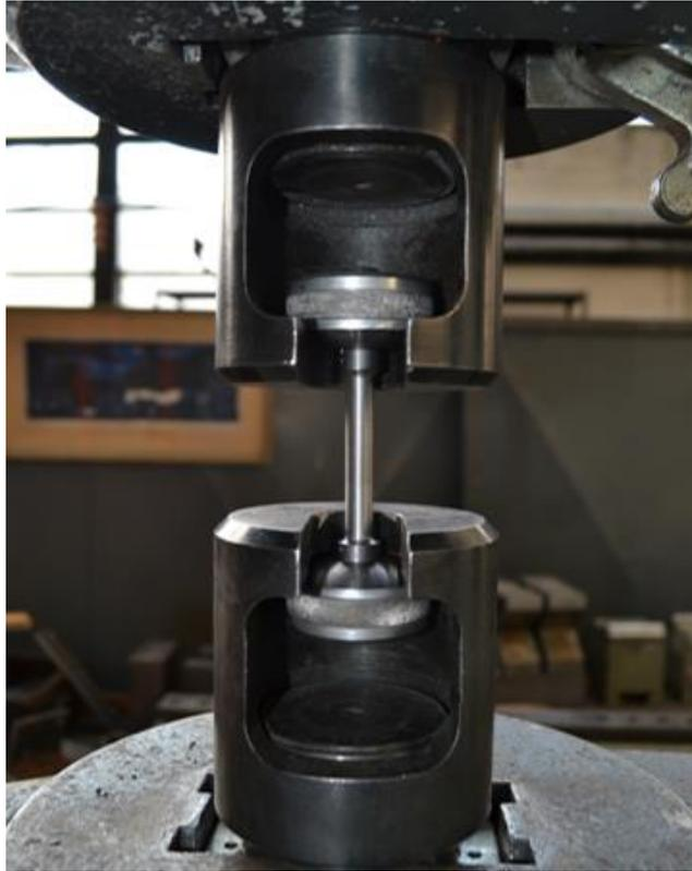
Figure 8: Tensile test procedure
