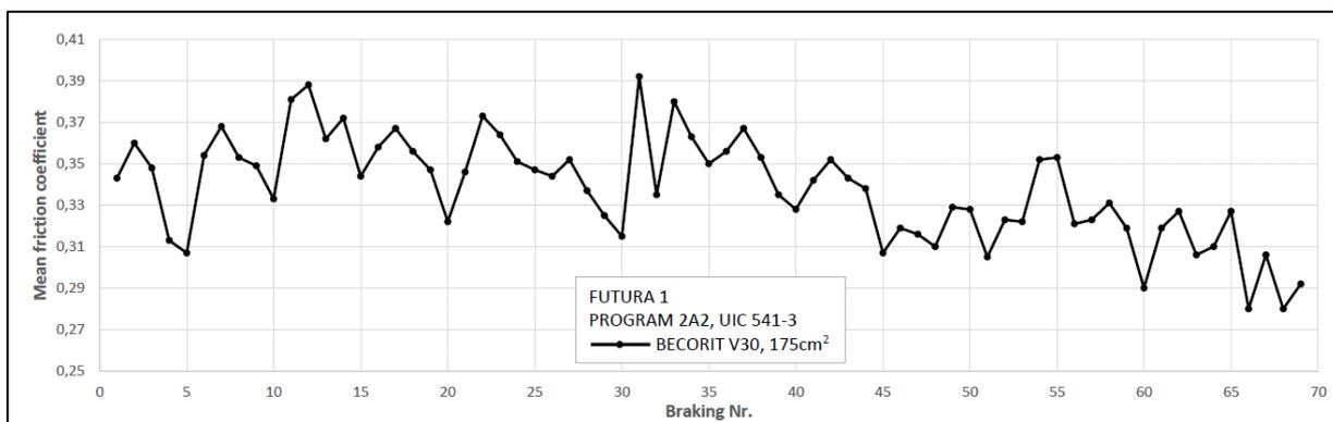
Figure 31: Friction coefficient of 1<sup>st</sup> prototype (Program 2A2)
