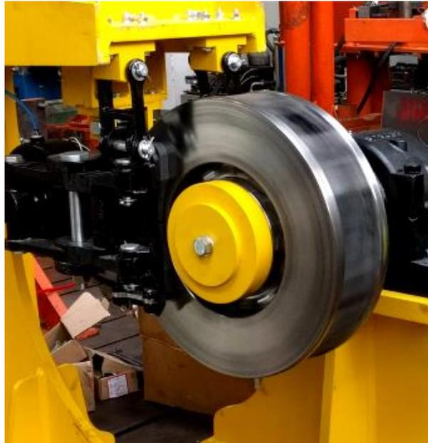
Figure 21: DRFB disc test bench
