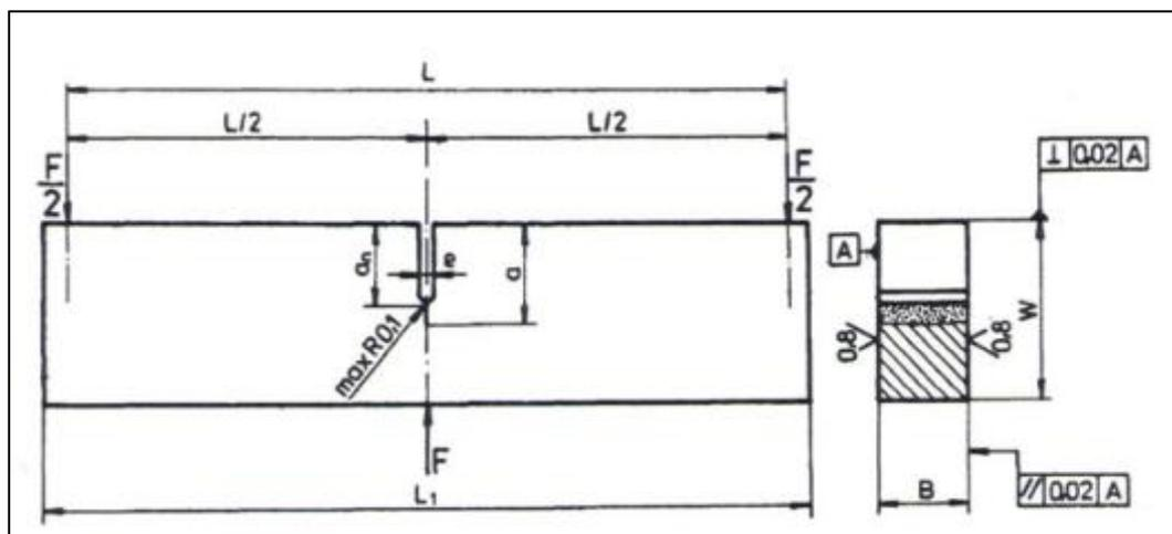
Figure 6: Shape and dimensions of fracture toughness samples
