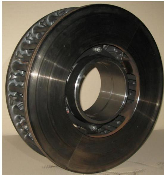
Figure 65: 4<sup>th</sup> prototype DRFB disc
