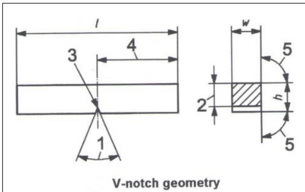
Figure 5: Shape and dimensions of Charpy test samples
