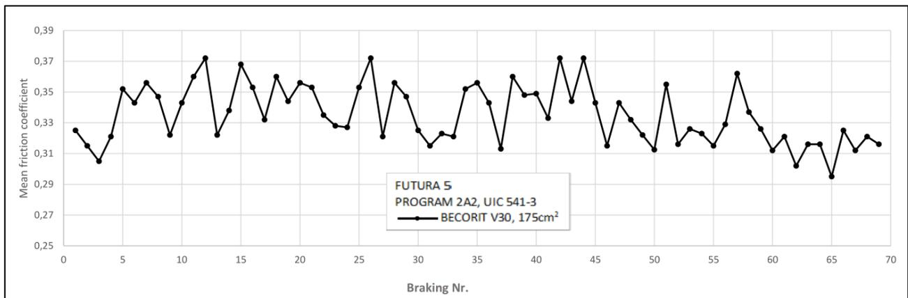
Figure 81: 5<sup>th</sup> prototype friction coefficient (Program 2A2)
