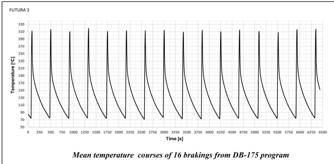
Figure 56: Temperatures of DRFB disc during DB-175 test
