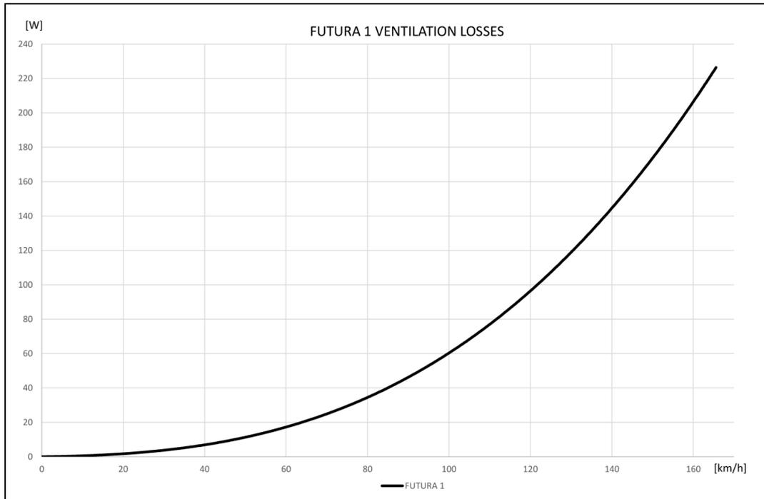
Figure 32: Ventilation losses for 1<sup>st</sup> prototype
