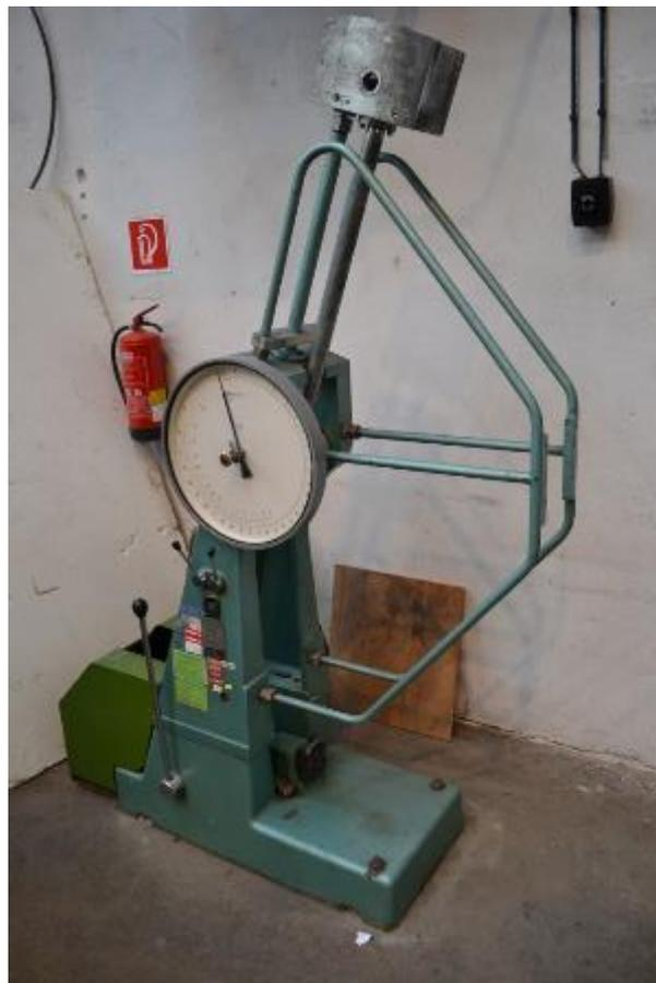
Figure 16: Charpy test machine
