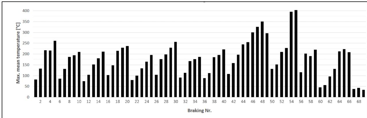
Figure 25: Temperatures of disc during 2A2 test program
