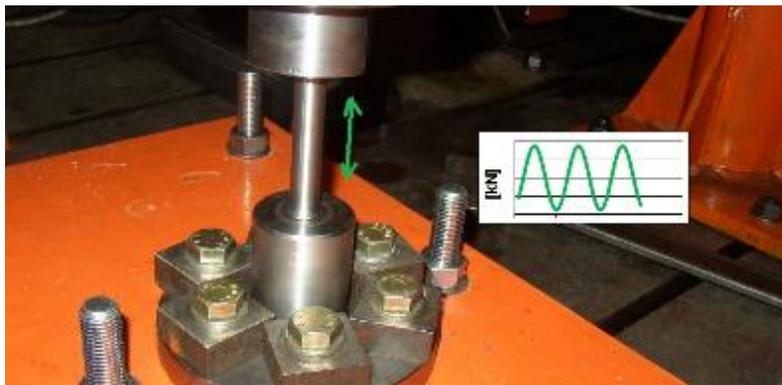
Figure 13: Fatigue test process
