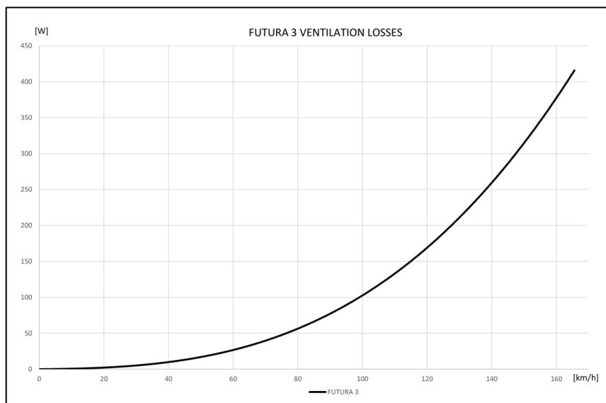
Figure 60: 3<sup>rd</sup> prototype ventilation losses
