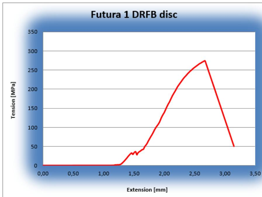
Figure 9: Graphic progress of 1<sup>st</sup> prototype DRFB disc crown tensile test
