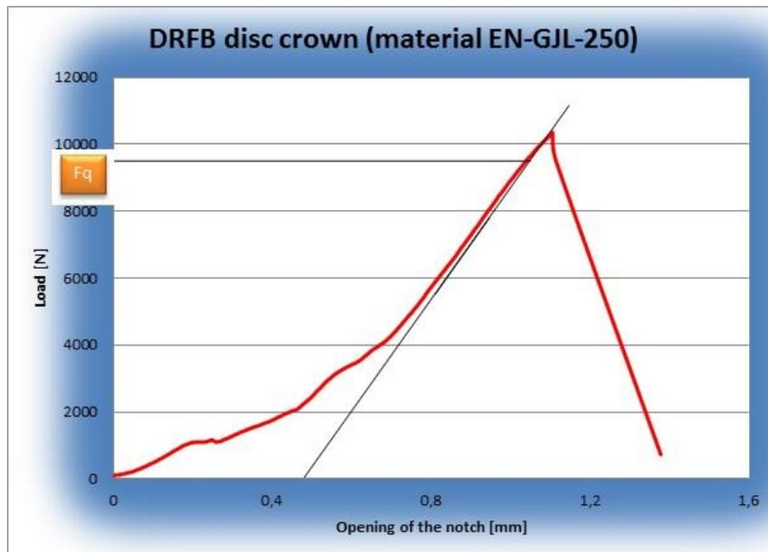
Figure 20: DRFB disc crown graphic fracture toughness progress
