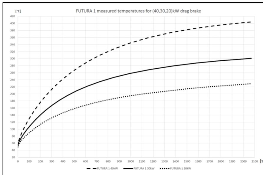
Figure 26: Temperatures of disc during heat dissipation test
