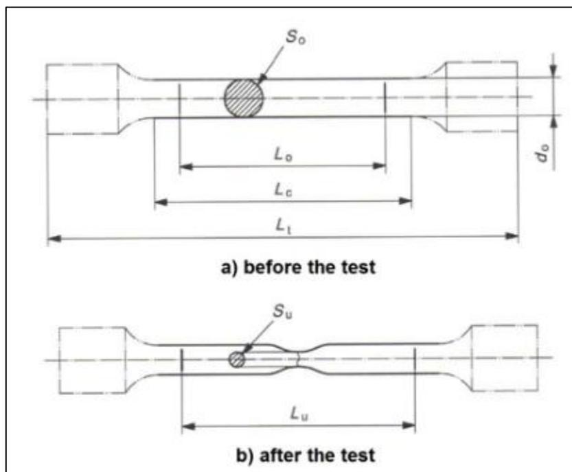
Figure 4: Shape and dimensions of tensile test samples
