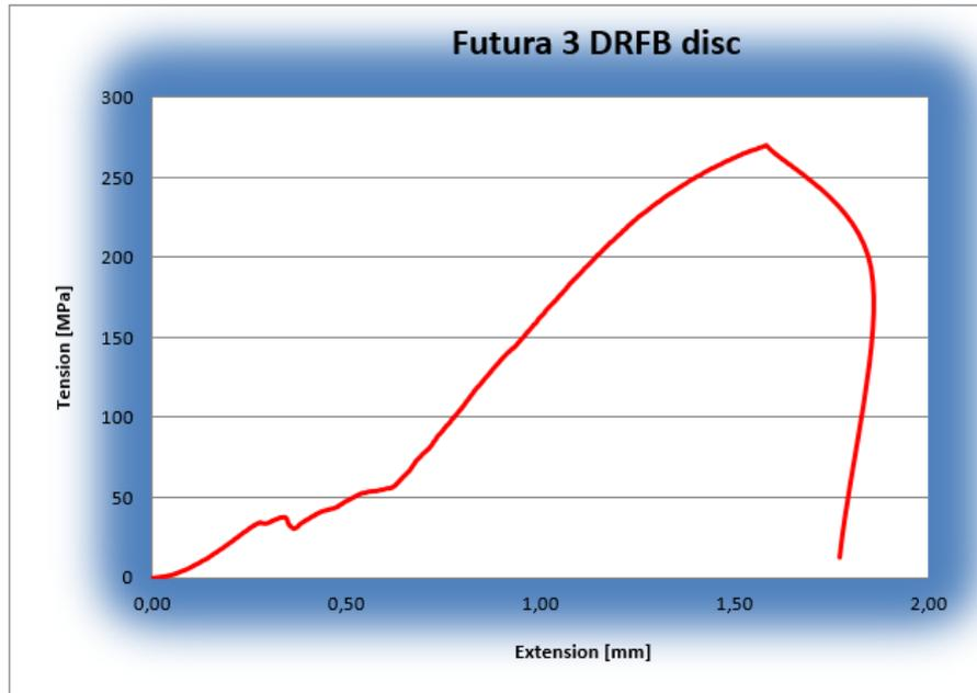
Figure 49: Graphic progress of 3<sup>rd</sup> prototype DRFB disc crown tensile test
