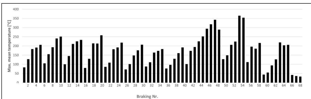
Figure 66: Temperatures of DRFB disc during 2A2 test program
