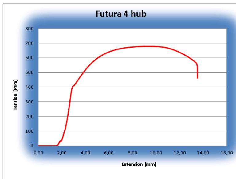
Figure 62: Graphic progress of 4<sup>th</sup> prototype DRFB disc hub tensile test
