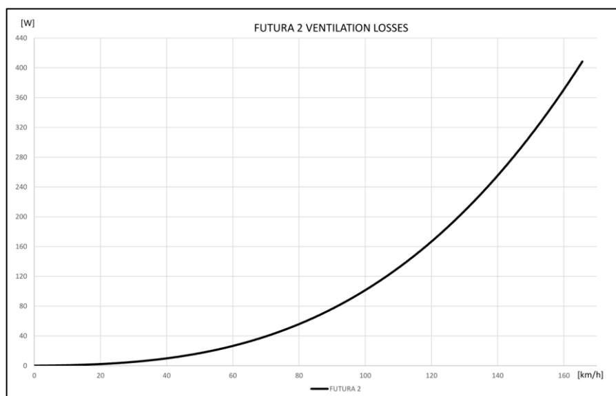
Figure 48: 2<sup>nd</sup> prototype ventilation losses
