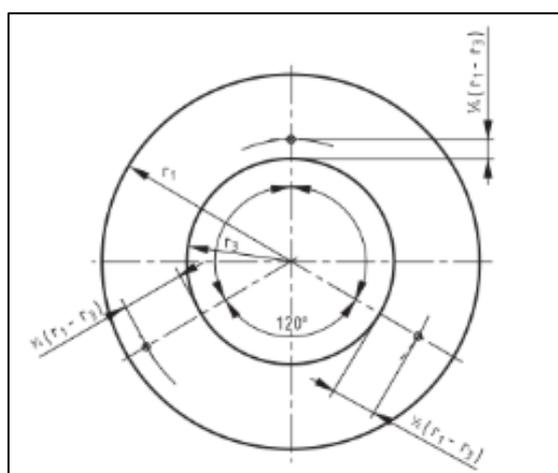
Figure 23: Position of temperature sensors
