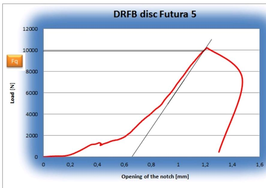
Figure 74: DRFB disc crown graphic fracture toughness progress
