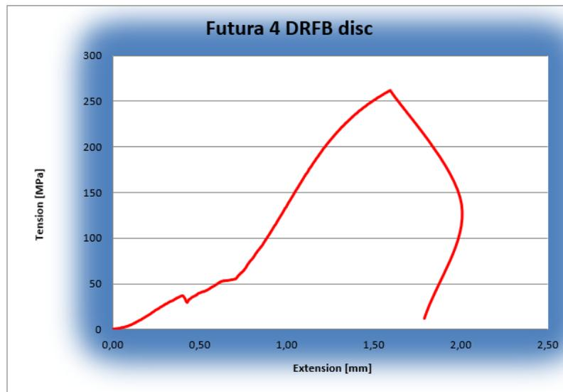
Figure 61: Graphic progress of 4<sup>th</sup> prototype DRFB disc crown tensile test
