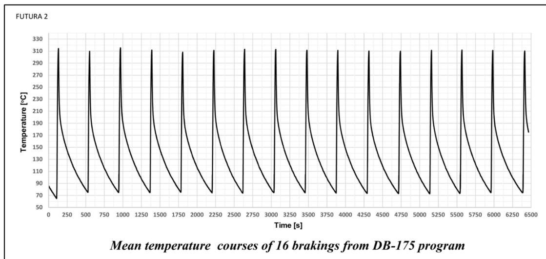
Figure 44: Temperatures of DRFB disc during DB-175 test
