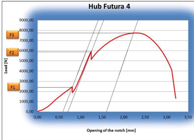
Figure 63: DRFB disc hub graphic fracture toughness test progress
