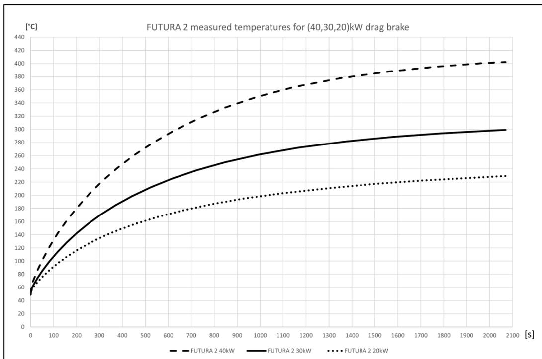
Figure 43: Temperatures of disc during heat dissipation test
