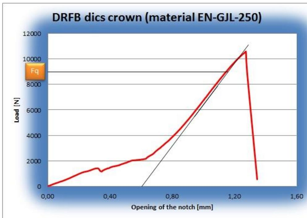
Figure 39: DRFB disc crown graphic fracture toughness progress
