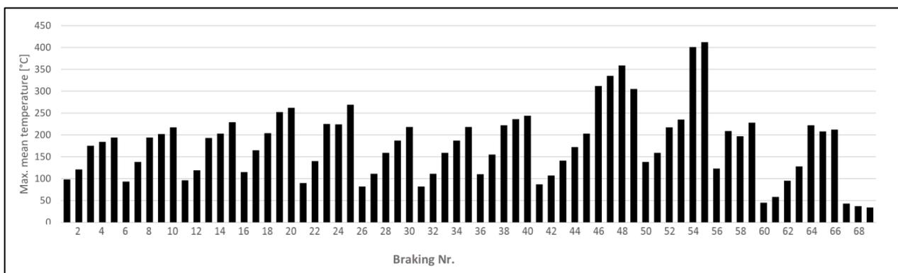
Figure 76: Temperatures of DRFB disc during 2A2 test program
